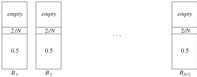
Figure 10.23 Next fit packing for 0.5, 2/N , 0.5, 2/N , 0.5, 2/N , ...
